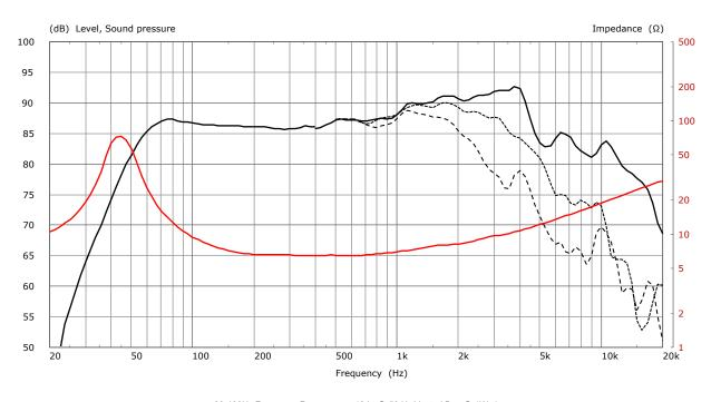
20-400Hz Frequency Response on 18 Lt @ 50 Hz Vented Box @ 1W, 1m 400-20000Hz Frequency Response on IEC Baffle (DIN 45575) @ 25cm, normalized to SPL 1W,1m Dotted line off-axis Frequency respone at 30°,60° - Free Air Impedance Measurement in Anechoic Chamber
